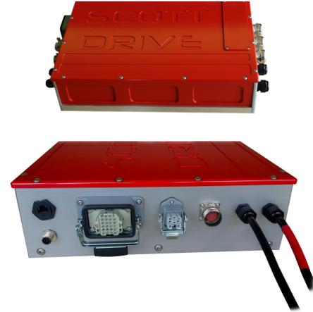
The Scott Drive family of AC Motor controllers is designed for easy integration into existing vehicles or for new OEM applications. With support for both Permanent Magnet (PM) and AC Induction (ACIM) motors the SD300 can provide up to 600 Arms of motor current from bus voltages up to 800V DC bus. Using the latest technology and high quality Automotive grade components the SD300 represents exceptional value and reliability for three Phase Motor control applications up to ~400kVA.
